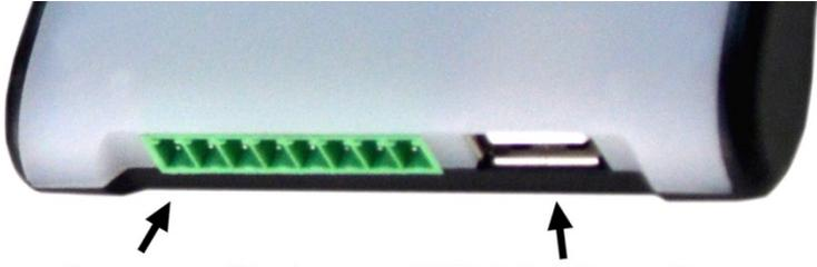
**Data Connector Pin 1**      **USB 2.0 A Type Connector**
