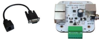
The cable adapter can be easily extended to the required length using regular Ethernet 8-wire cables.
