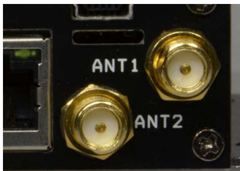
Figure 1: Sargas RFID Antenna Ports
