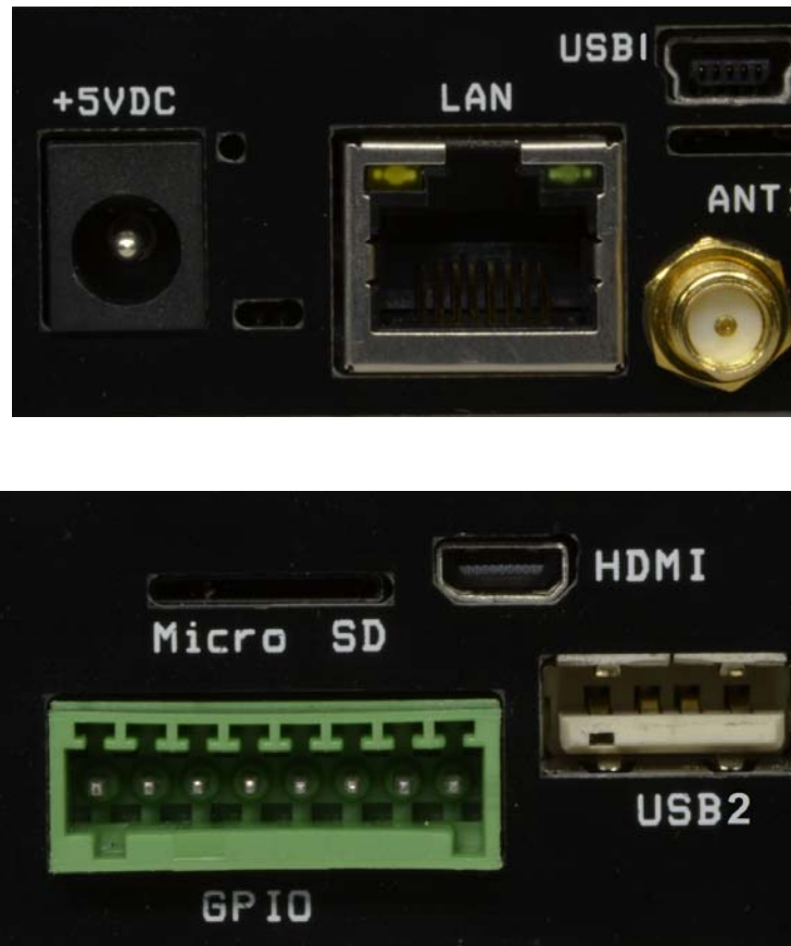
Figure 2: Sargas Digital and Power Connectors
