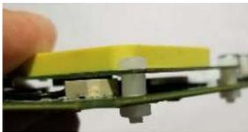
6. Use the nylon stand-offs to affix the feet at the 4 corners of the board as shown below, with the screw on top and the stand-off on the bottom. This will prevent components from shorting out on the surface below the board if that surface is conductive.
