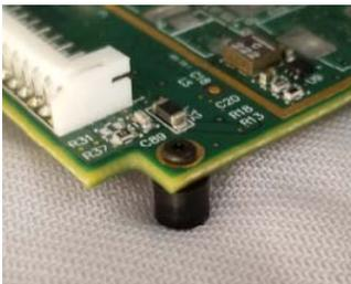
7. Attach the USB cable to the 13-pin connector on the board. Make sure the side of the connector faces up (as shown below), with the wires entering the connector as shown.
