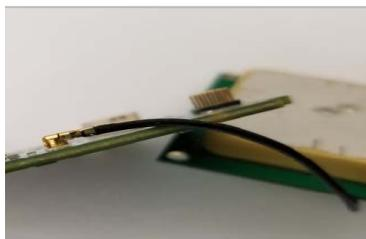
4. Rotate the antenna and cable above the board until the RF cable is oriented as shown below. Any other orientation of antenna to the board will cause the components on the bottom of the antenna to interfere with those on the top of the board.
